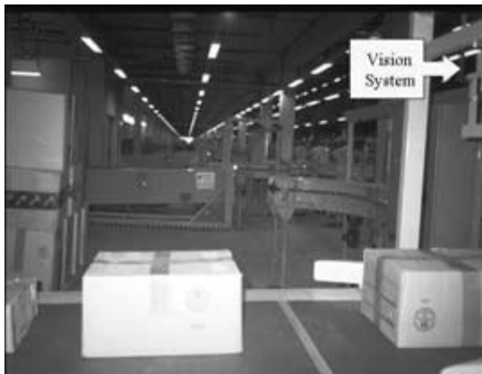
FIGURE 9-19 Vision system used in automated receiving inspection.
